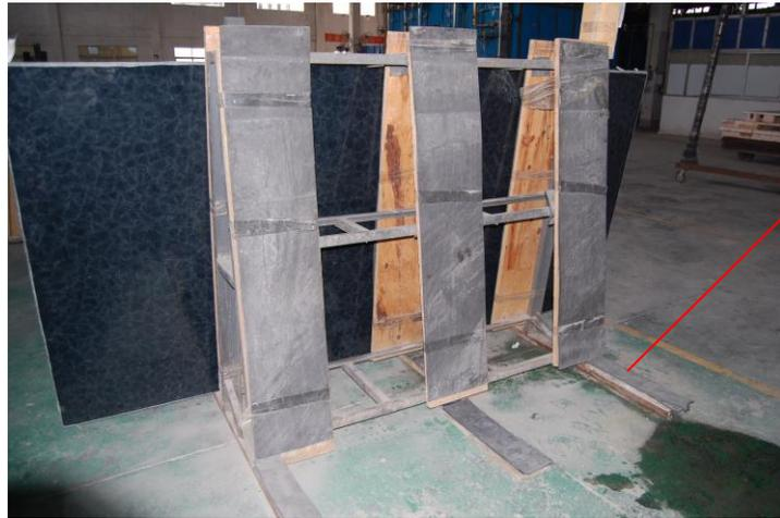
Backside and bottom of A frame must have soft material and wide board with soft material to support.
