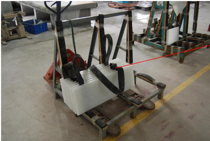
Separate each piece of GlassTech slabs with softy materials as it will not easy crash and broken.
